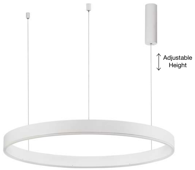
MOTIF - 9190755 · 3000K Triac Dimmable 9530211 · 2700-6000K Changing CCT & Dimming Sandy White Aluminium & Acrylic LED 60 Watt 4165Lm 230 Volt IP20 D: 100 H: 200 cm
