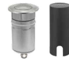
No 4285400 LED 3W • 161Lm 3000K • IP 67 Beam Angle 25° • CRI>80
